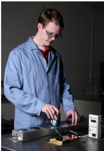
The emissivity was tested according to ASTM C1371, "Test Method for Determination of Emittance of Materials near Room Temperature Using Portable Emissometers." This method takes a random sampling of each material and, using a small tabletop device, emits heat onto the product with a heat sink below and measures the amount of infrared heat that emits through.
