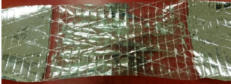
**If results like these arose in the field, the product would need to be uninstalled and replaced with a product that would still work as a radiant barrier.**
