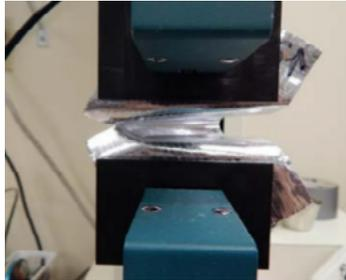
Since the Direct-Metalized Woven Fabric product is not a stiff, laminated, but rather a thin, pliable fabric, we had concerns about it stretching (rather than tearing) under the stress of the test and throwing off the results. To make sure we were getting a fair comparison between products, we also included a strength test specifically designed for non-laminated fabrics, ASTM D4533, “Standard Test Method for Trapezoid Tearing Strength of Geotextiles.”
