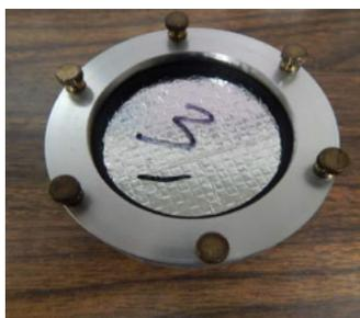
Procedure A of the ASTM E96 test method seals a sample of the material over the top of a small cup, which has been partially filled with a moisture-absorbing desiccant at a steady atmospheric temperature and humidity level. The samples are then removed, and the moisture absorbed through the tested material into the desiccant is measured. ASTM E96 gives this measurement both in grams per square meter per 24 hours, and more simply, in units called perms.
